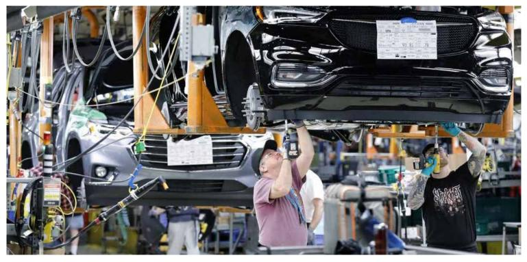
The automotive industry involves a lot of underbody shot work to tighten bolts or drive screws on the underside of vehicles. Performing these tasks manually, especially on an assembly line, means an employee is holding a tool at or above shoulder level repeatedly over long periods of time. The employee must also deal with tool torque and contorting to work on hard-to-reach places when doing underbody shots.
